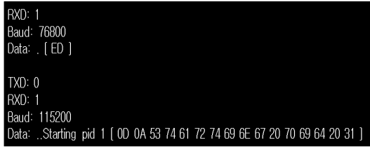
Fig. 7. Identify baudrate using jtagulator
